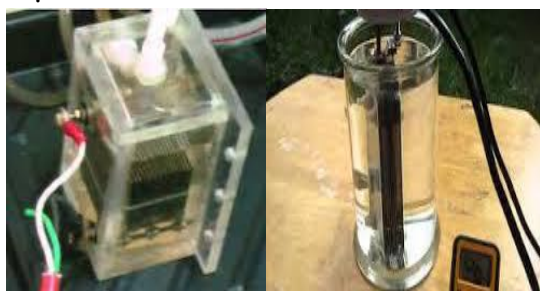
Gambar 2. Generator HHO tipe Wet Cell (Silaen and Kawano, 2014)
